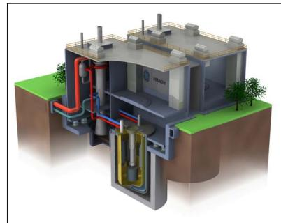
Figure 2: PRISM Reactor power block used to produce electricity from spent nuclear fuel.
