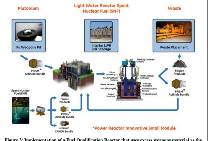
Figure 3: Implementation of a Fuel Qualification Reactor that uses excess weapons material as the initial core and recycled light water reactor spent fuel in subsequent operations.
